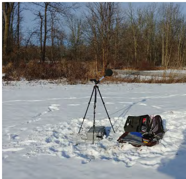
Figure 1-7 Location 2 - Winter, Sound Level Meter Example Setup
