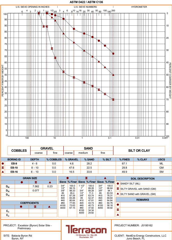
GRAIN SIZE: USCS 1 J5195162 EXCELSIOR (BYRON) WITH LAB WORK GPJ TERRACON\_DATATEMPLATE. GDT 12/10/19 REPORT. LABORATORY TESTS ARE NOT VALID IF SEPARATED FROM ORIGINAL
