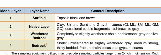
1. The sampling equipment utilized may preclude sampling particles larger than 2-inch in dimension. Rock fragments and split-spoon sampler refusal was encountered at some locations (5 borings) within the depths explored, indicating the presence of possible cobbles and boulders.
